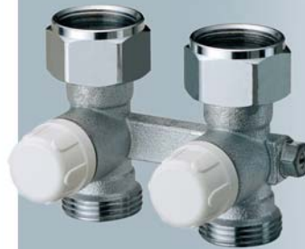
Art. 1421 SINGLE-DOUBLE PIPE angled valve. Adjustable by-pass. Connections: 3/4 EUROKONUS Centre line between ports: 50 mm
