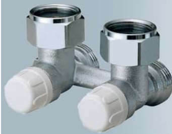
Art. 1421 SINGLE-DOUBLE PIPE angled valve. Adjustable by-pass. Connections: 3/4 EUROKONUS Centre line between ports: 50 mm
