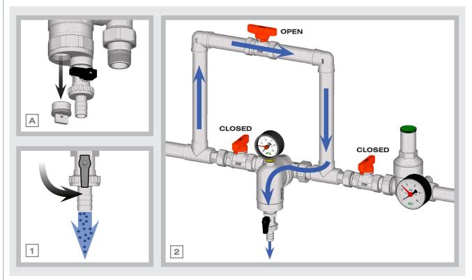
For a more thorough cleaning, once closing the ball valves (**Fig. 3**), unscrew the bottom body of the strainer using a wrench and remove the cartridge (**Fig. 4**). Once removed all the impurities on the filter mesh, reposition the cartridge at the bottom of the strainer and re-tighten it (**Fig. 5**).
