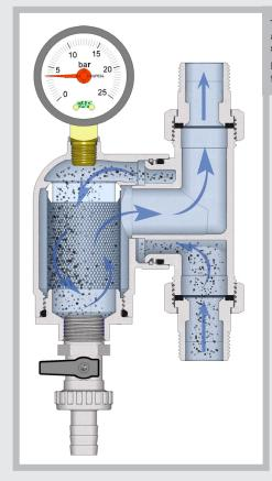
The incoming water follows a guided path entering the filtering net from above and then moves in a radial direction, getting rid of impurities. The particles thus stick to the net or fall down, accumulating near the drain valve.
